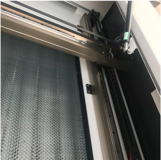
2/ Adopt high speed Linear motion guide, ensuring the laser head is moving smoothly, fast and stable. Small cutting kerf, high cutting speed and accuracy guarantee the equipment's precision and lifetime.
